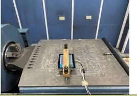
Random Vibration Test: Y axis/ Mechanical Shock Test: ±Y axis
