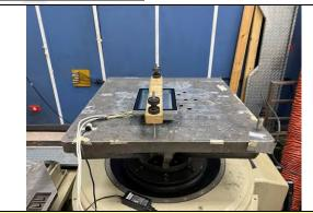
Random Vibration Test: Z axis/ Mechanical Shock Test: ±Z axis
